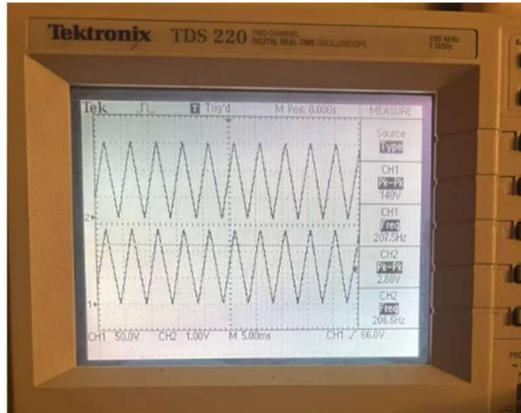
2.43 uF Capacitive Load with 207Hz Triangle Wave Input
