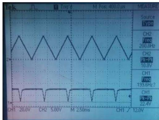
High Voltage Disable ON (ENA-RIGHT-PIN=+24V), the output is 24V with 0-10V triangle wave input
